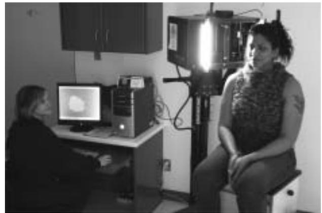
*3D Laser Scanning Station in the Medical Modeling Research Laboratory (MMRL). The laser scanner allows non-invasive capturing of surface features in 3D. Stephanie White-Downey, Clinical Assistant, COMPRU and a person being scanned.*
